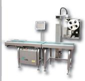
The WIL-700 is a long scale variant of the modular WI-700 with the infeed and scale decks at 650mm. This allows the processing of products up to 475mm long at a fixed speed of up to 37ppm. The WIL-700 has a 15kg/5g scale capacity.
